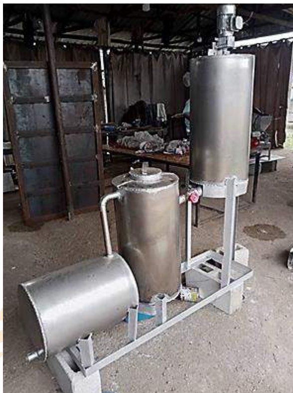
Figure 01: Fabricated Simultaneous Saccharification and fermentation Skid Unit
